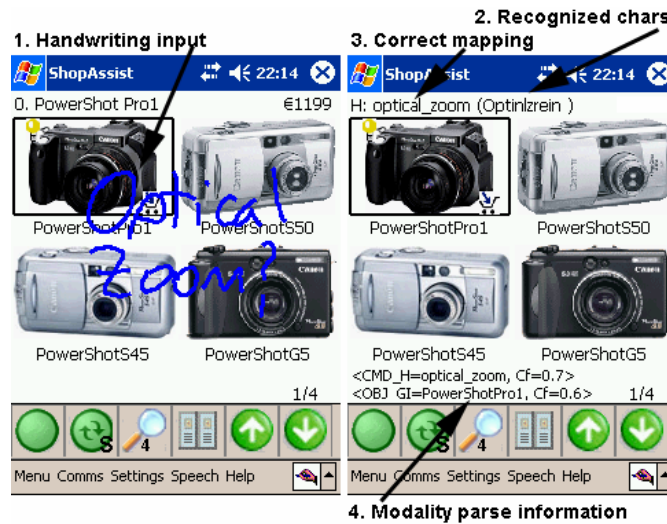
Fig. 3. An example of how a handwriting event (1) is recognized by the character recognizer (2), and then mapped to a valid grammar entry (3). Also note the summarized modality recognition results (4)
