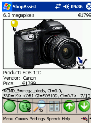
Fig. 4. The circled parse information shows a mapping of the modalities speech (S) and intra gesture (GI) to that of the uni-modal language elements command (CMD) and object (OBJ)
