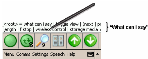
Fig. 6. Displayed as scrolling text, a visual “what can I say” can allow the user to access command functionality through stylus intra-gestures
