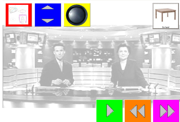
Figure 4: Multimedia user interface. Virtual control elements from left to right: device selector, channel selector, volume control, Play/Pause, Rewind, Forward.
