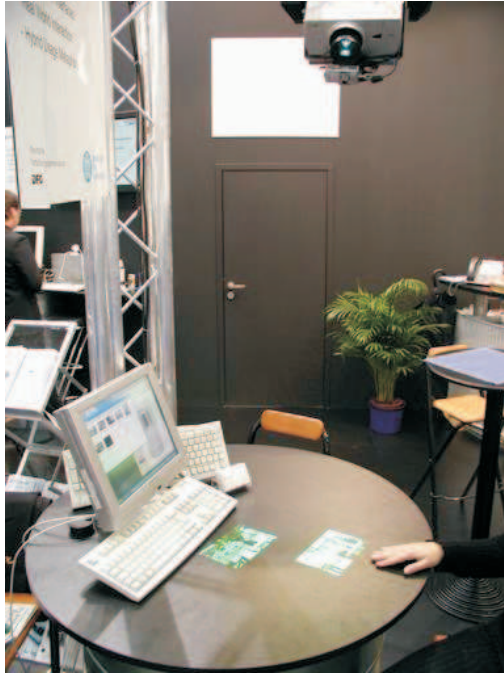
Figure 4. Wipe gesture recognition scenario: a selection of two images is displayed on the desk; the white surface on the wall is used for the slide show
